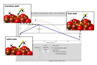
With combinations of different computational techniques, *MedeA Transition State Search* finds energy barriers of a multitude of diffusion pathways of atoms in solids, exemplified in the figure below for migration of Li cations in a battery cathode material.
